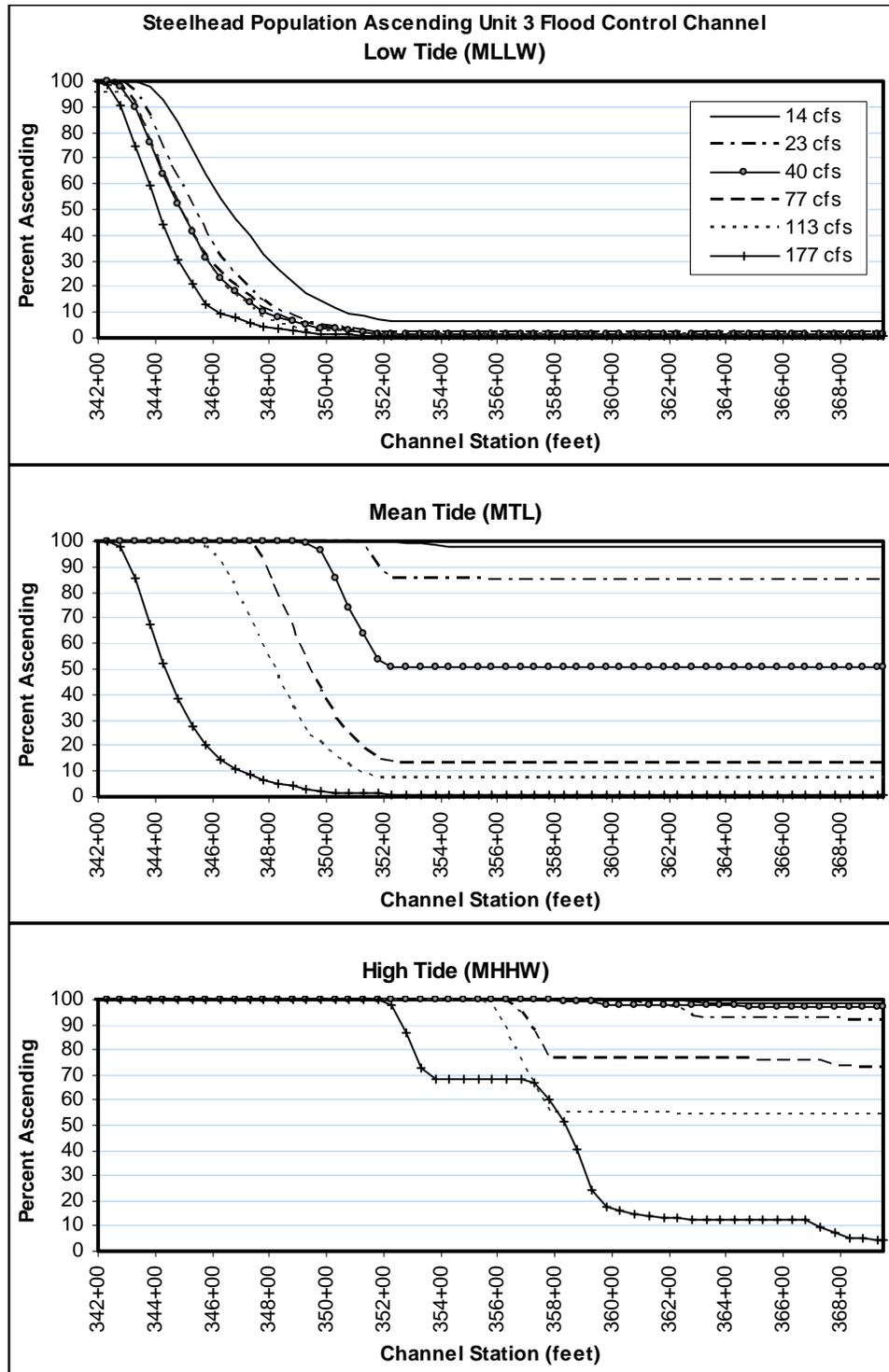
**Figure 5.3** – Existing steelhead passage conditions. Percent of individual adult steelhead from the population capable of reach the corresponding Unit 3 channel station at a given flow and tidal condition. The existing resting pools begin at Station 350+85.
