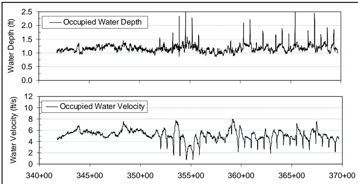
**Figure 5.2** – At 177 cfs and tidal conditions equal to MLLW, the “occupied” water velocities and depths encountered by the fish along its swimming route through Unit 3.
