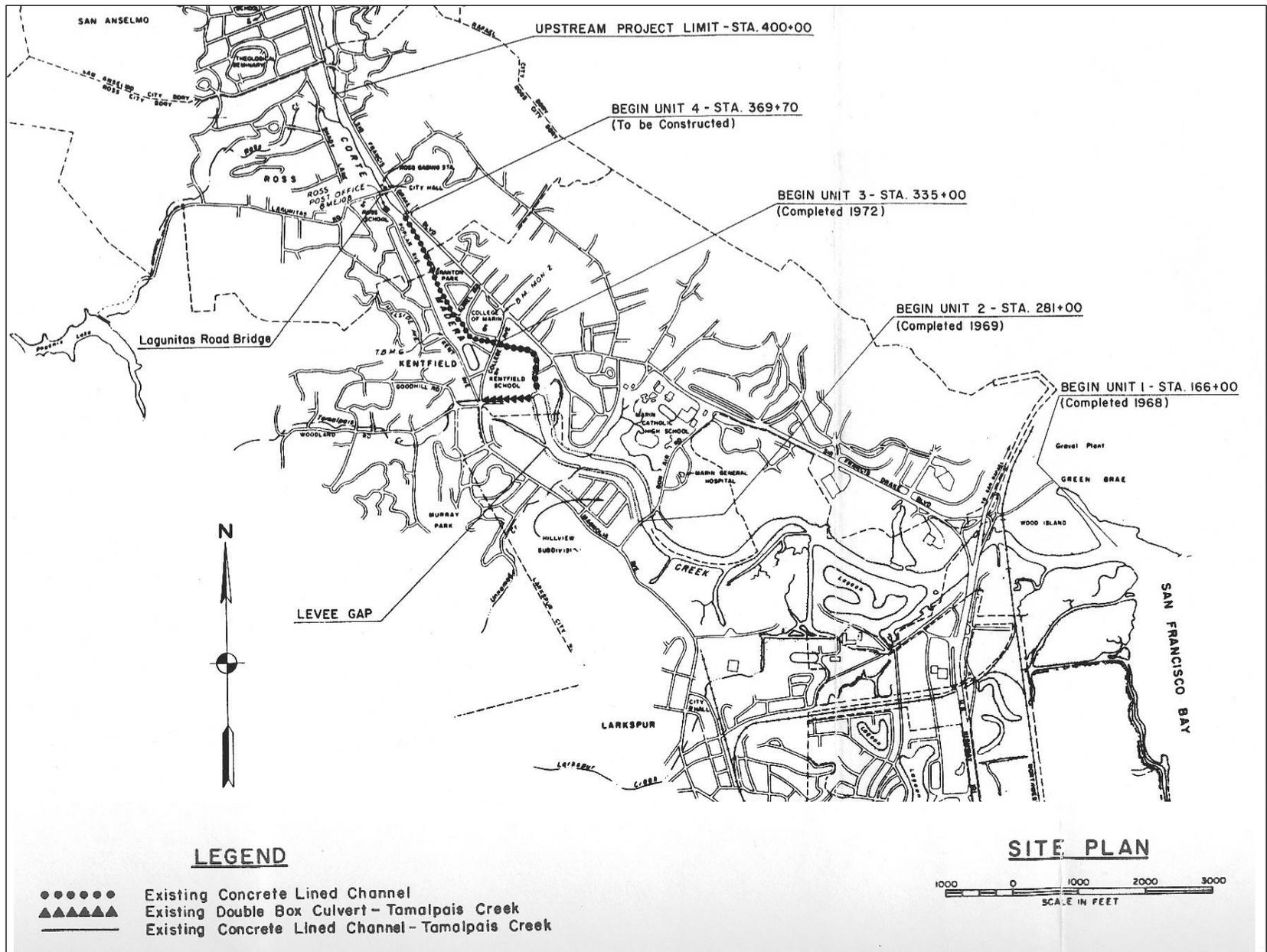
Figure 1.1 – Site map of the Corte Madera Creek Flood Control Channel, Units 1 through 4 (adapted from ACOE, 1989).
