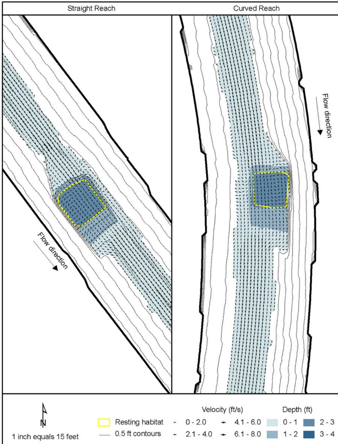
**Figure 6.20** – Alternative 3 water depth, water velocity field, and available resting habitat at the low passage design flow of 114 cfs.
