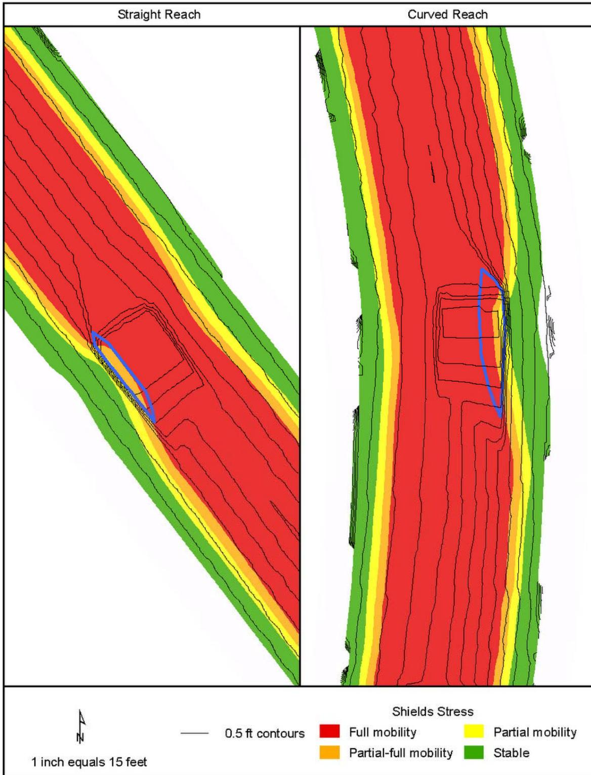
**Figure 6.23** – Alternative 3 predicted mobility of streambed material at the 1.5 year return flow of 1,383 cfs.
