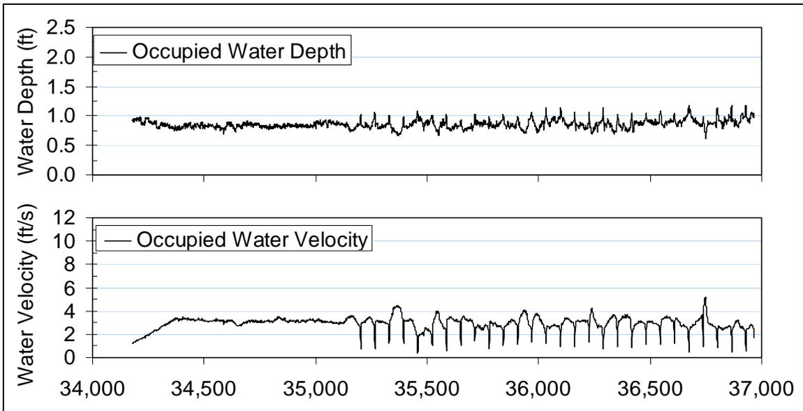
Fish occupied water depths and velocities at 14 cfs.
