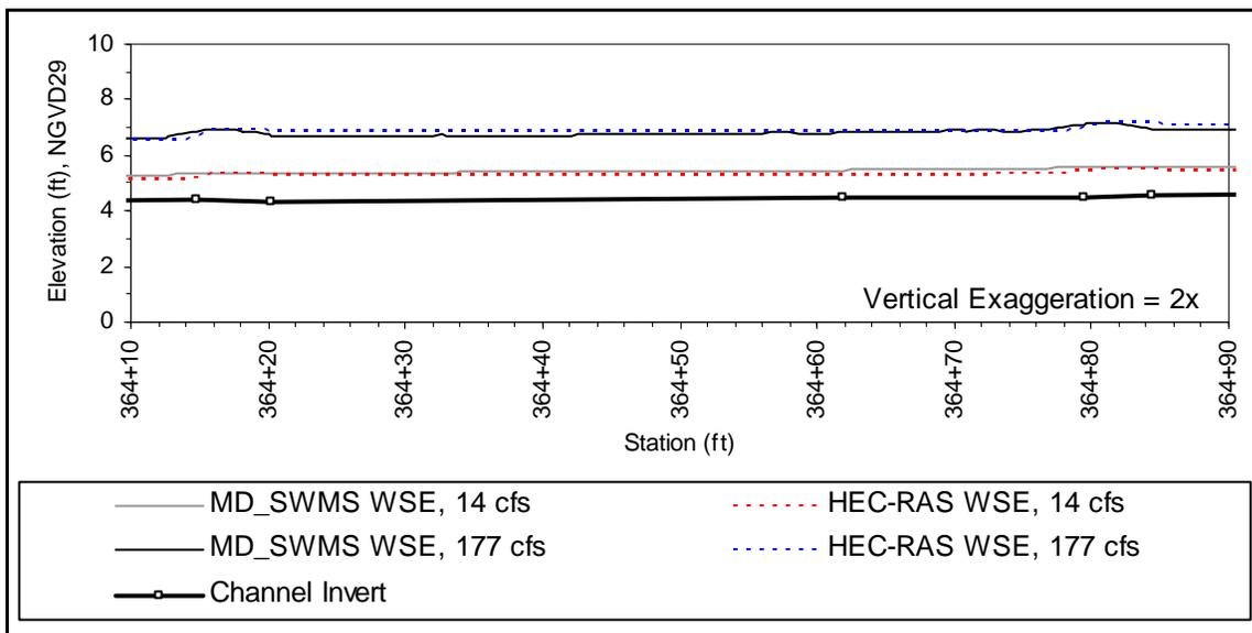
**Figure 4.2** - HEC-RAS and MD\_SWMS predictions of water surface elevation at 14 cfs and 177 cfs at two pools in model reach, Unit 3.
