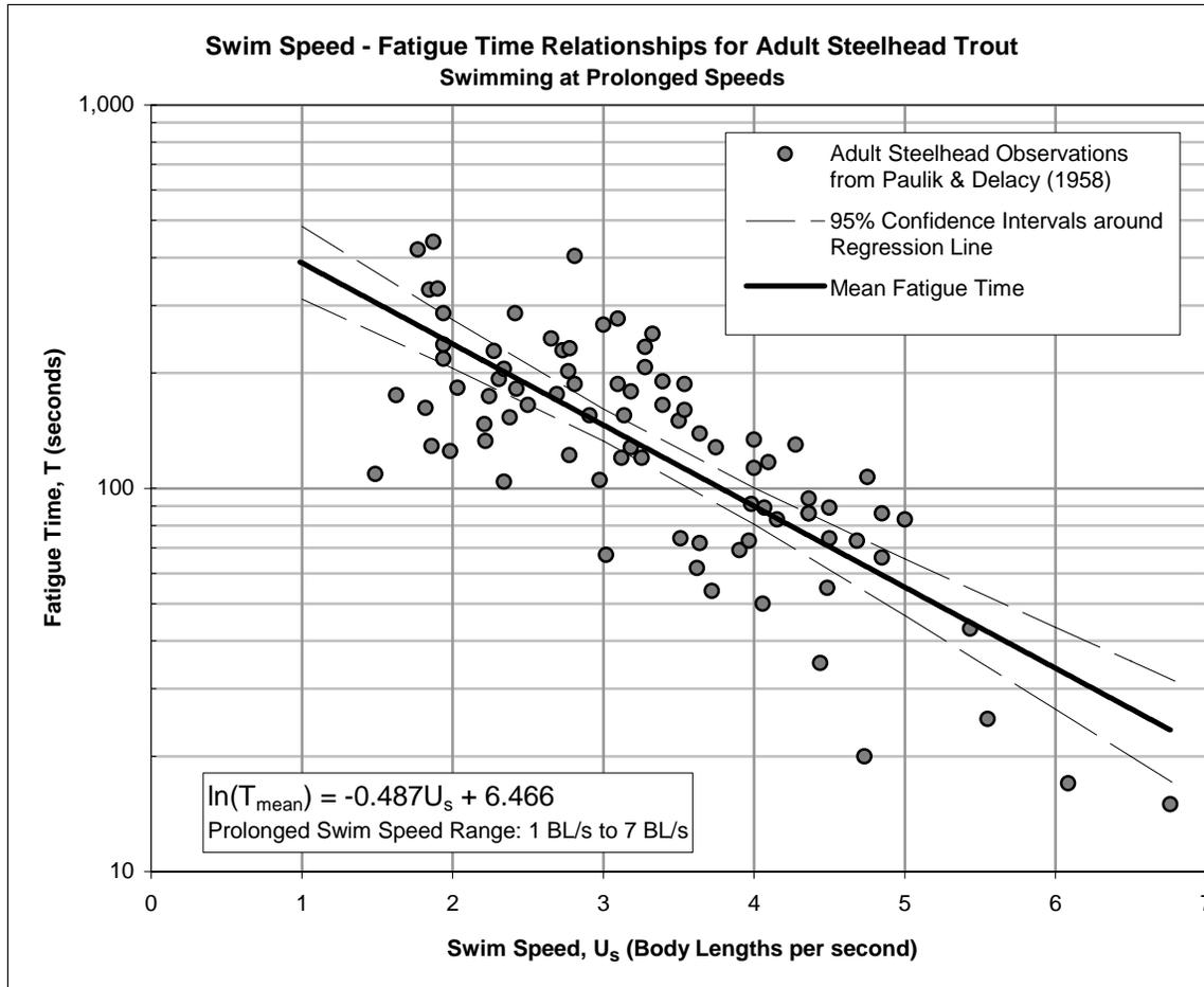
**Figure 4.4**—Relationship of swim speed verses time to fatigue for steelhead trout swimming at prolonged speeds, developed from data presented in Paulik and Delacy (1958).
