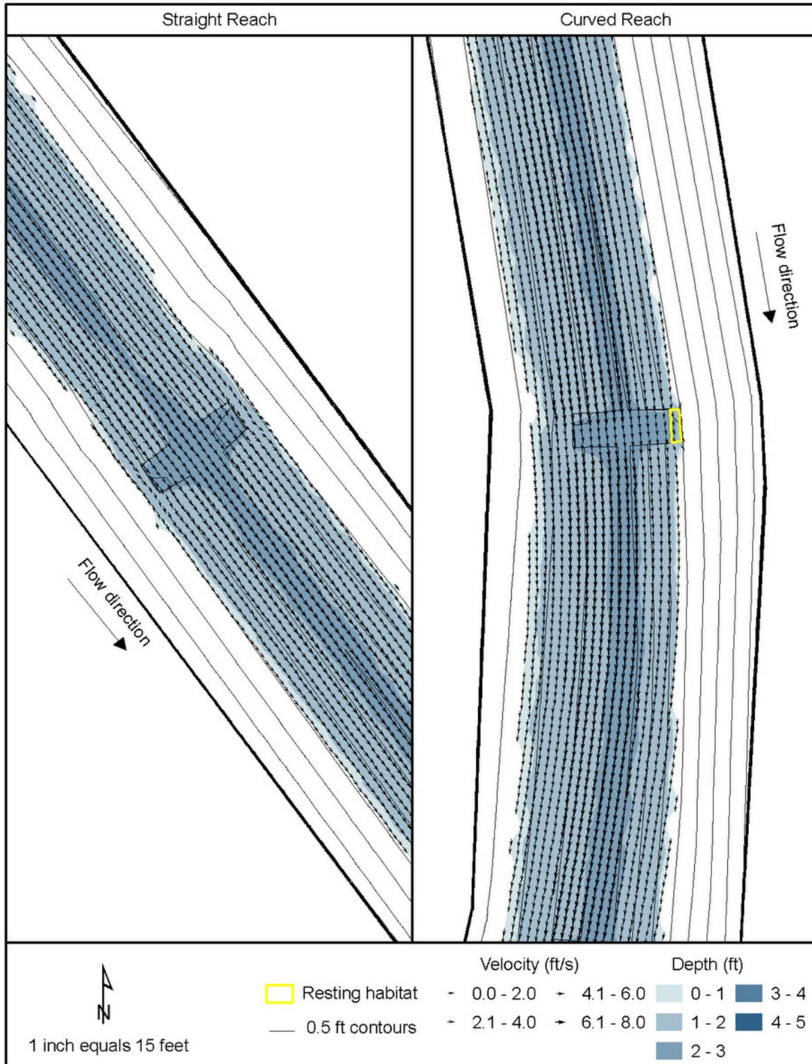
**Figure 6.3** – Existing water depth and velocity field at the high passage design flow of 177 cfs. Resting habitat is not large enough for a fish to hold.
