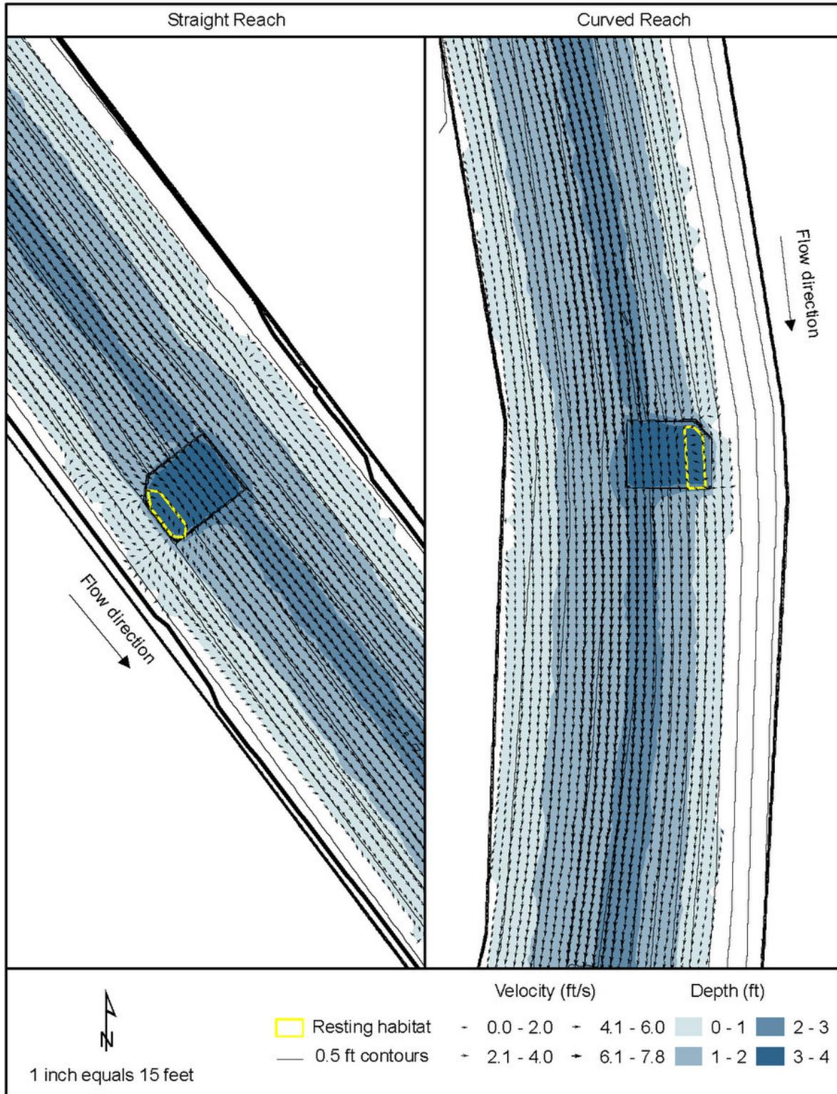
**Figure 6.15** – Alternative 2 water depth, water velocity field, and available resting habitat at high passage design of 177 cfs.
