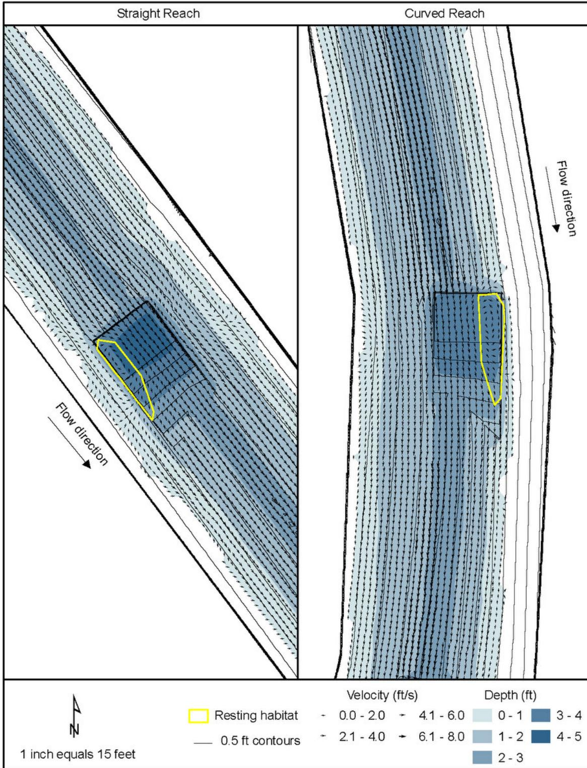
**Figure 6.9** – Alternative 1 water depth, water velocity field, and available resting habitat at high passage design of 177 cfs.
