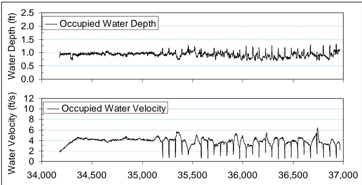
Fish occupied water depths and velocities at 23 cfs.
