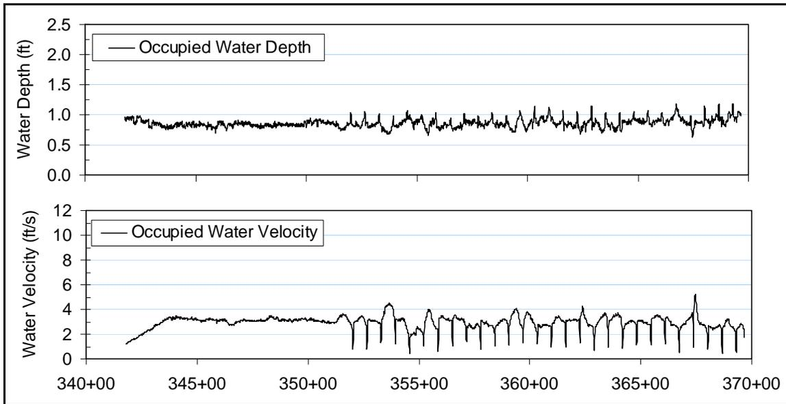
**Figure 5.1** – At 14 cfs and tidal conditions equal to MLLW, the “occupied” water velocities and depths encountered by the fish along its swimming route through Unit 3.
