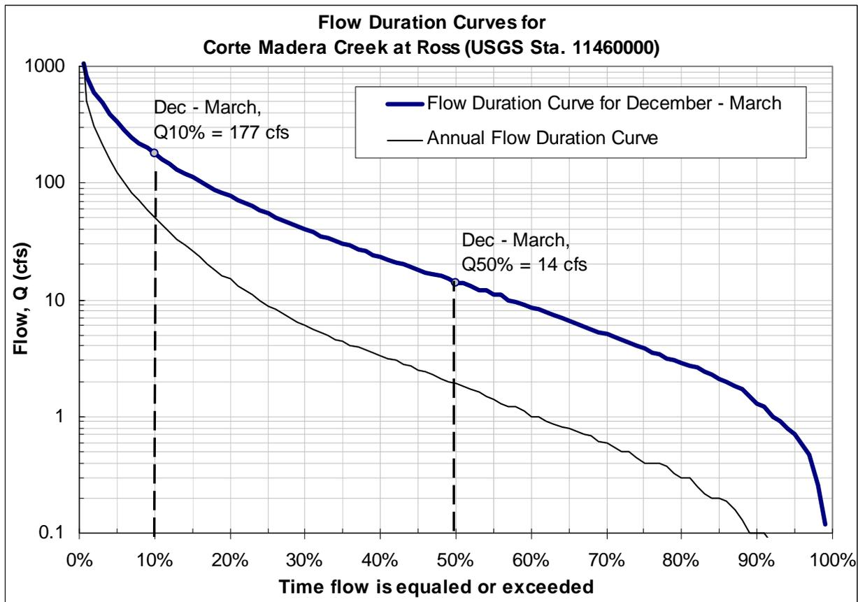
**Figure 3.1** – Annual and steelhead migration period (November through March) flow duration curves for Corte Madera Creek, constructed using daily average flows recorded from 1951 to 1993 at the USGS gage at Ross.
