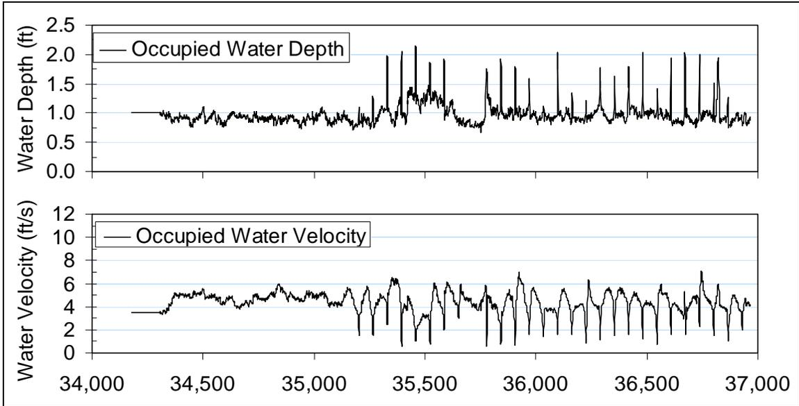
Fish occupied water depths and velocities at 113 cfs.
