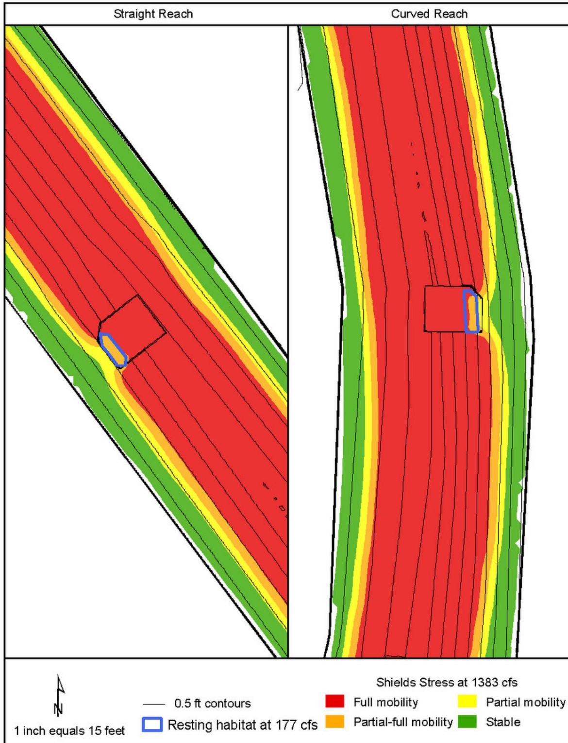
**Figure 6.17** – Alternative 2 predicted mobility of streambed material at the 1.5 year return flow of 1,383 cfs.
