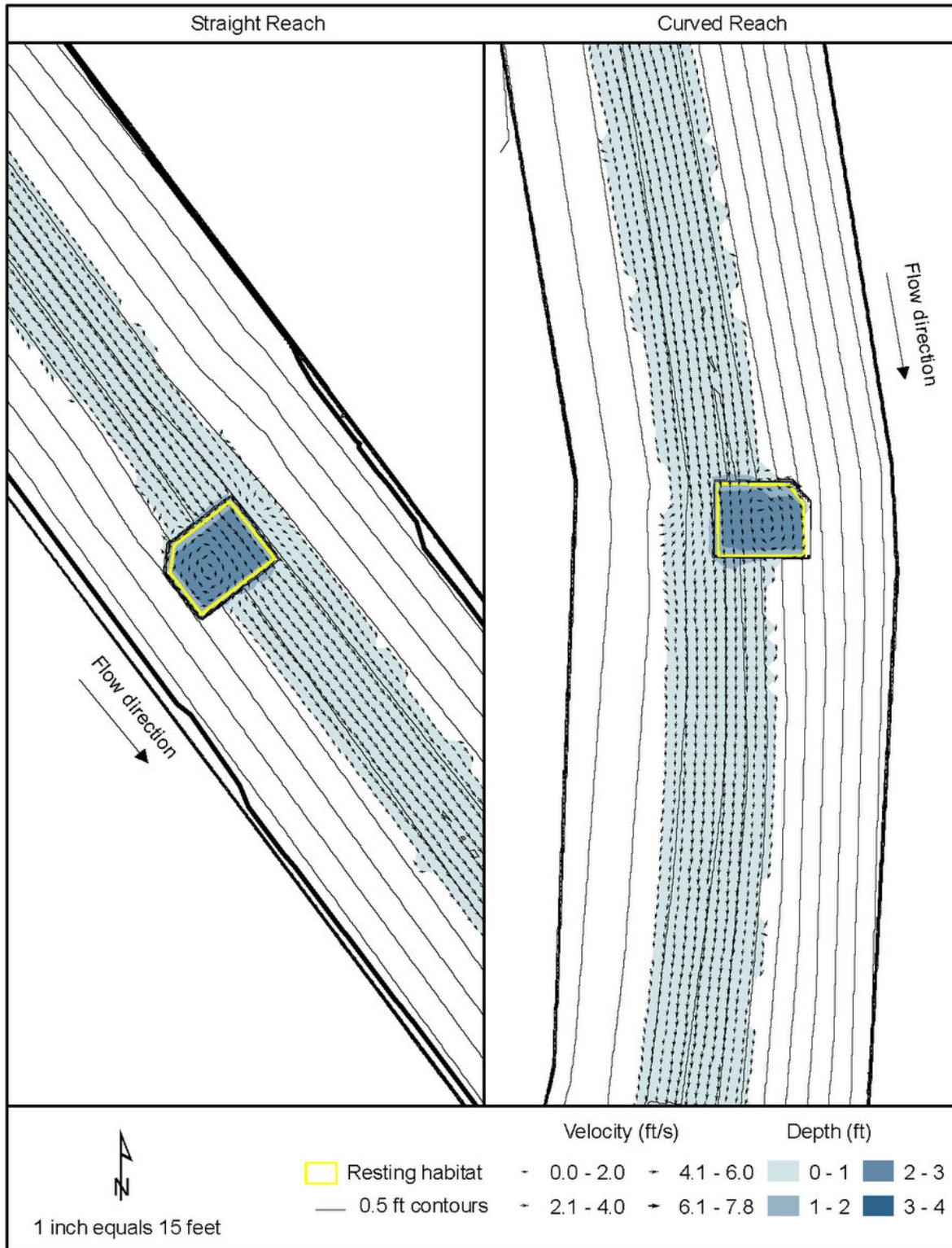
**Figure 6.14** – Alternative 2 water depth, water velocity field, and available resting habitat at the low passage design flow of 114 cfs.
