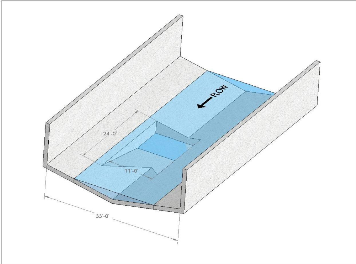
**Figure 6.6** – Isometric drawing of Alternative 1 resting pool.
