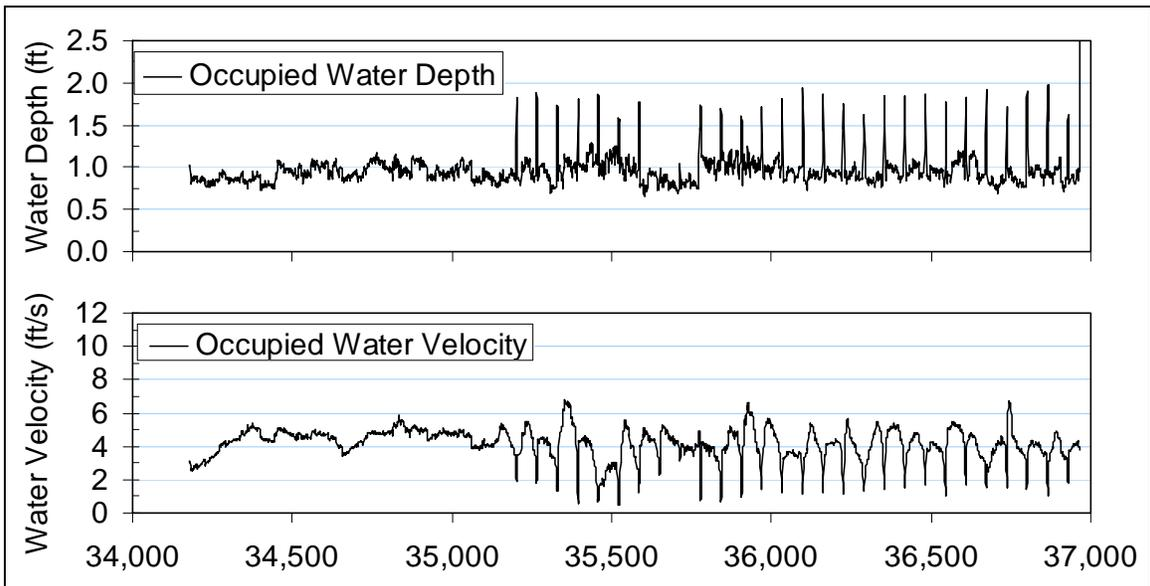
Fish occupied water depths and velocities at 77 cfs.
