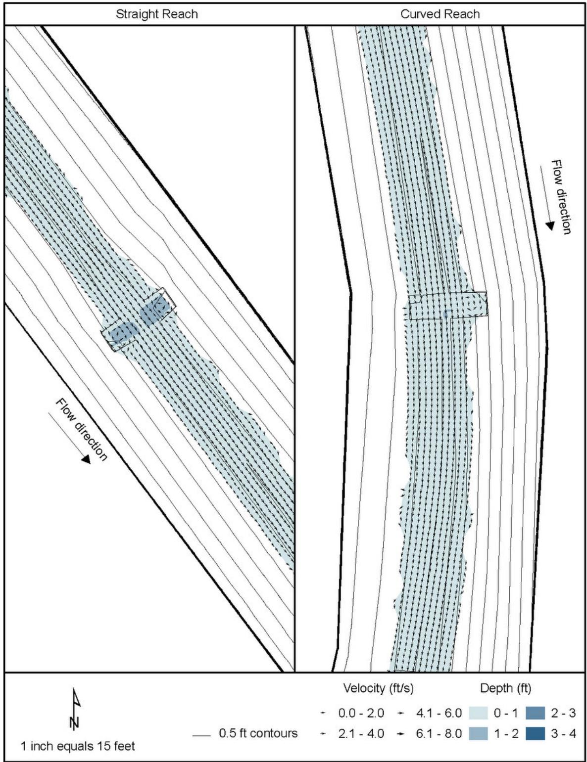
**Figure 6.2** – Existing water depth and velocity field at the low passage design flow of 14 cfs. No resting habitat exists due to low flow depths.
