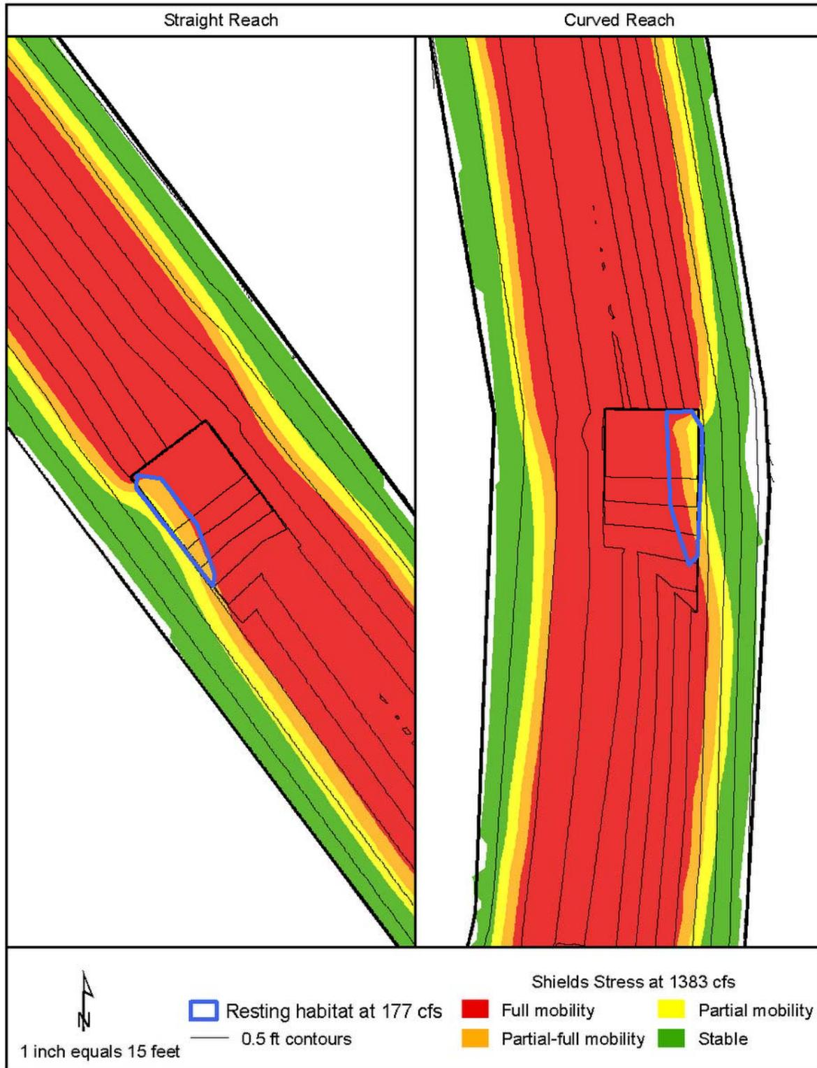
**Figure 6.11** – Alternative 1 predicted mobility of streambed material at the 1.5 year return flow of 1,383 cfs.
