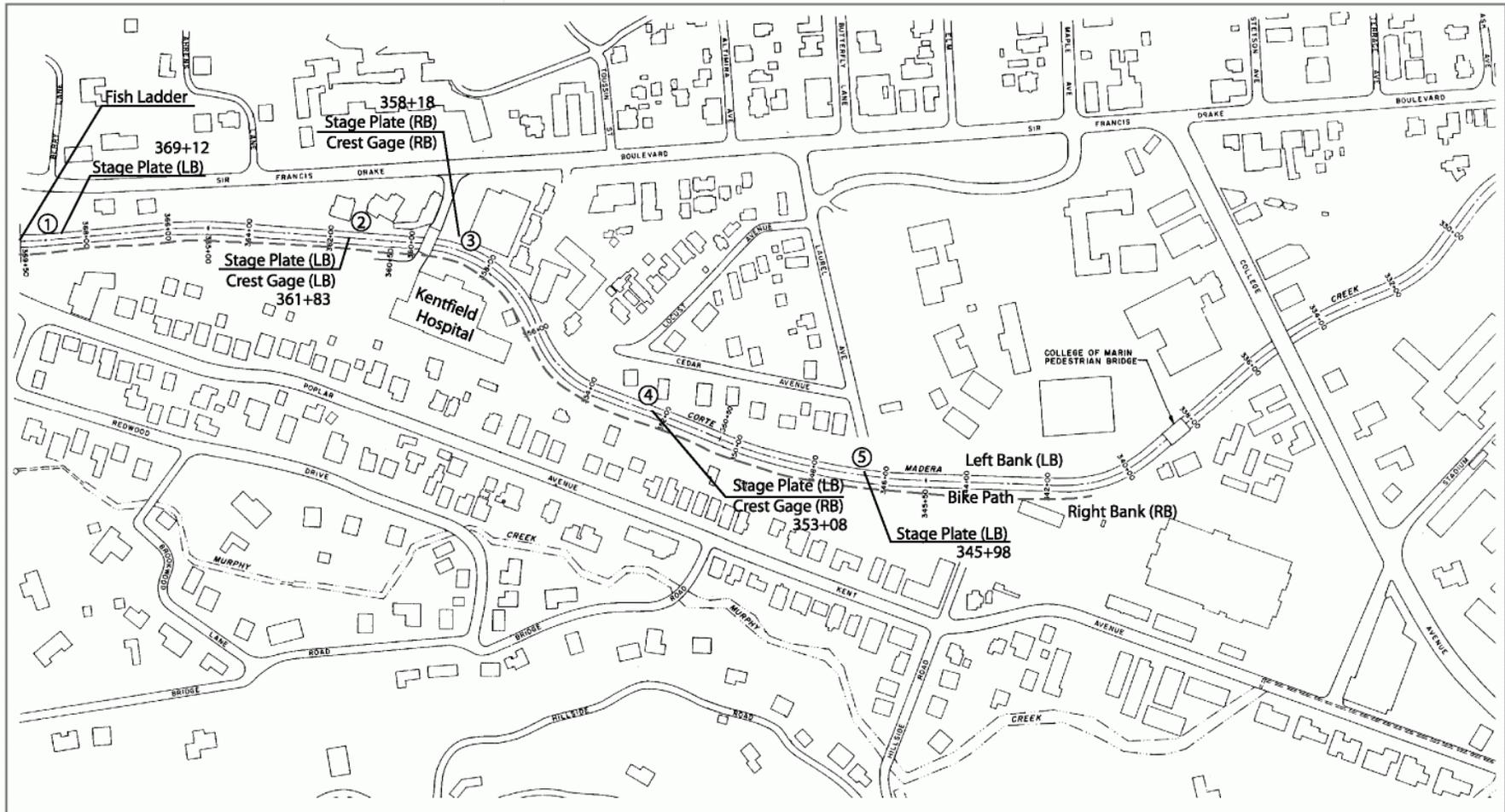
**Figure 2.1** – Location of monitoring stations 1 through 5 and associated stage plates and crest gages in Unit 3 (adapt from ACOE, 1989).
