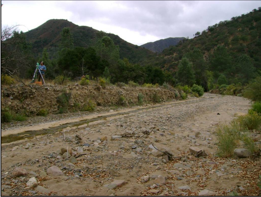
(STA 5+30) Looking downstream at aggraded reach downstream of removed dam.
