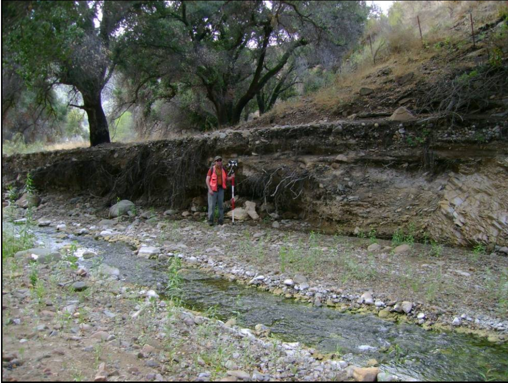
(STA 14+50) Looking downstream at exposed bedrock in incised and widened channel.
