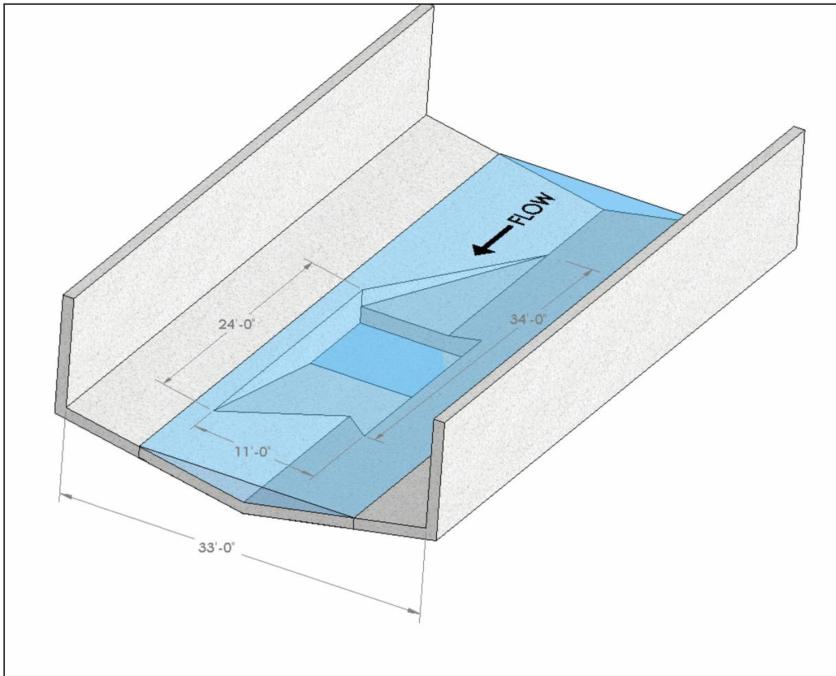
**Figure 6.18** – Isometric drawing of Alternative 2 resting pool.
