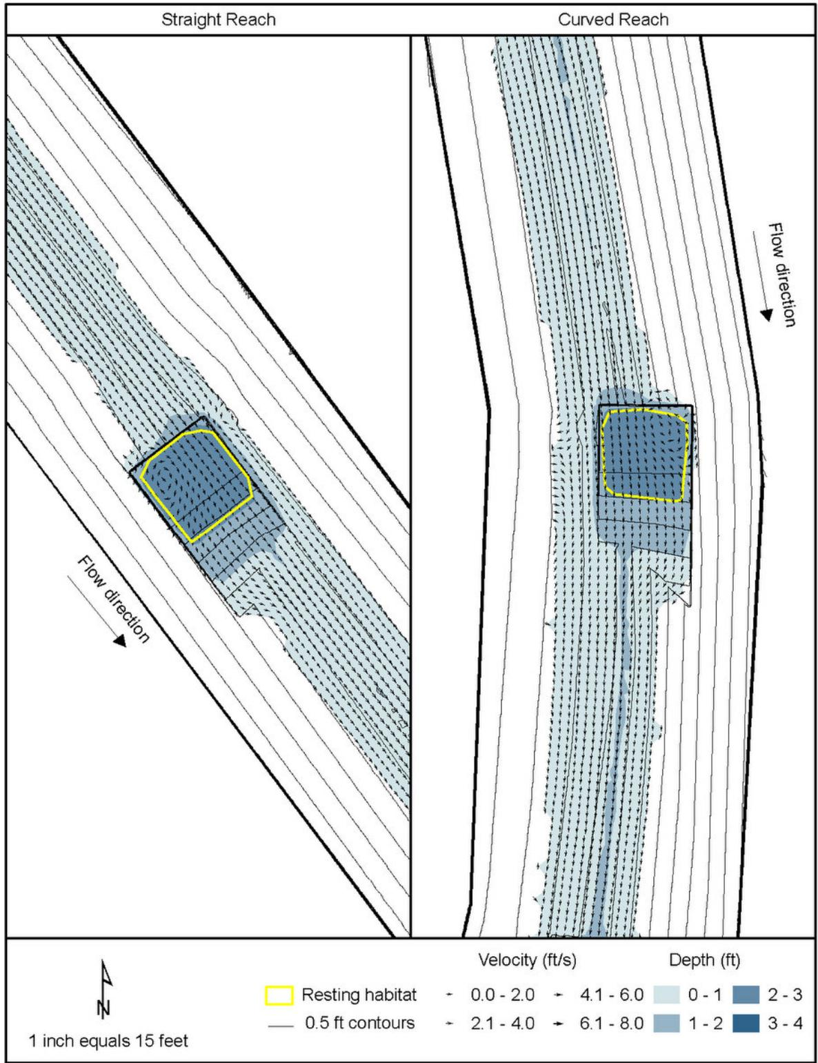
**Figure 6.8** – Alternative 1 water depth, water velocity field, and available resting habitat at the low passage design flow of 114 cfs.
