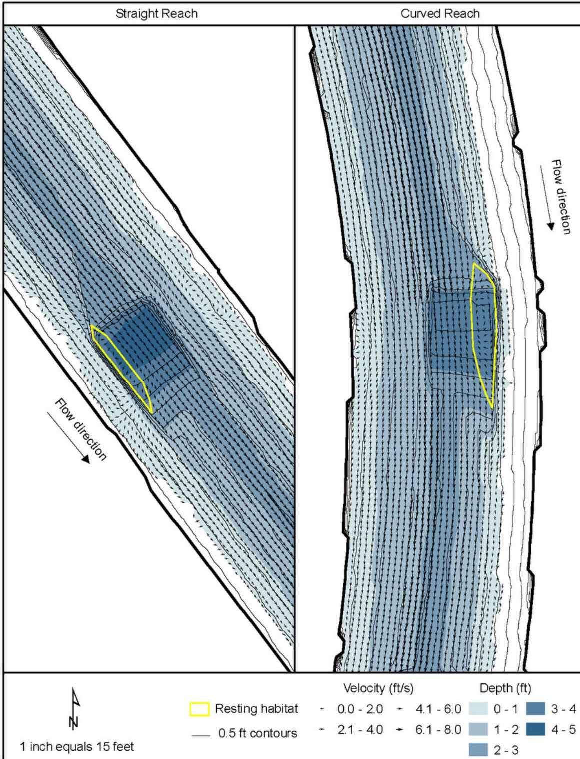
**Figure 6.21** – Alternative 3 water depth, water velocity field, and available resting habitat at high passage design of 177 cfs.
