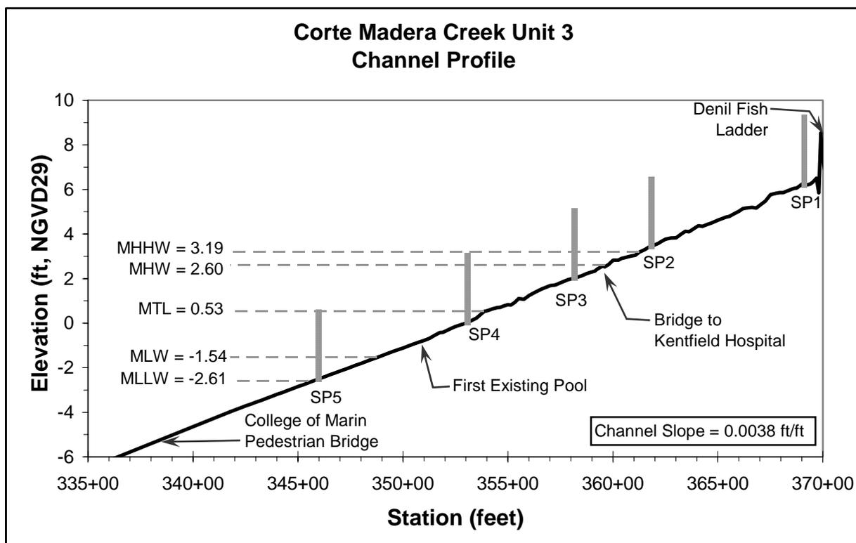
**Figure 1.2** – Profile of the channel invert in Unit 3. Tidal elevations and locations of the two bridge crossings, fish ladder and downstream most resting pool are noted on the profile. The location and overall height of the five stage plates (SP) installed as part of this project are also shown.
