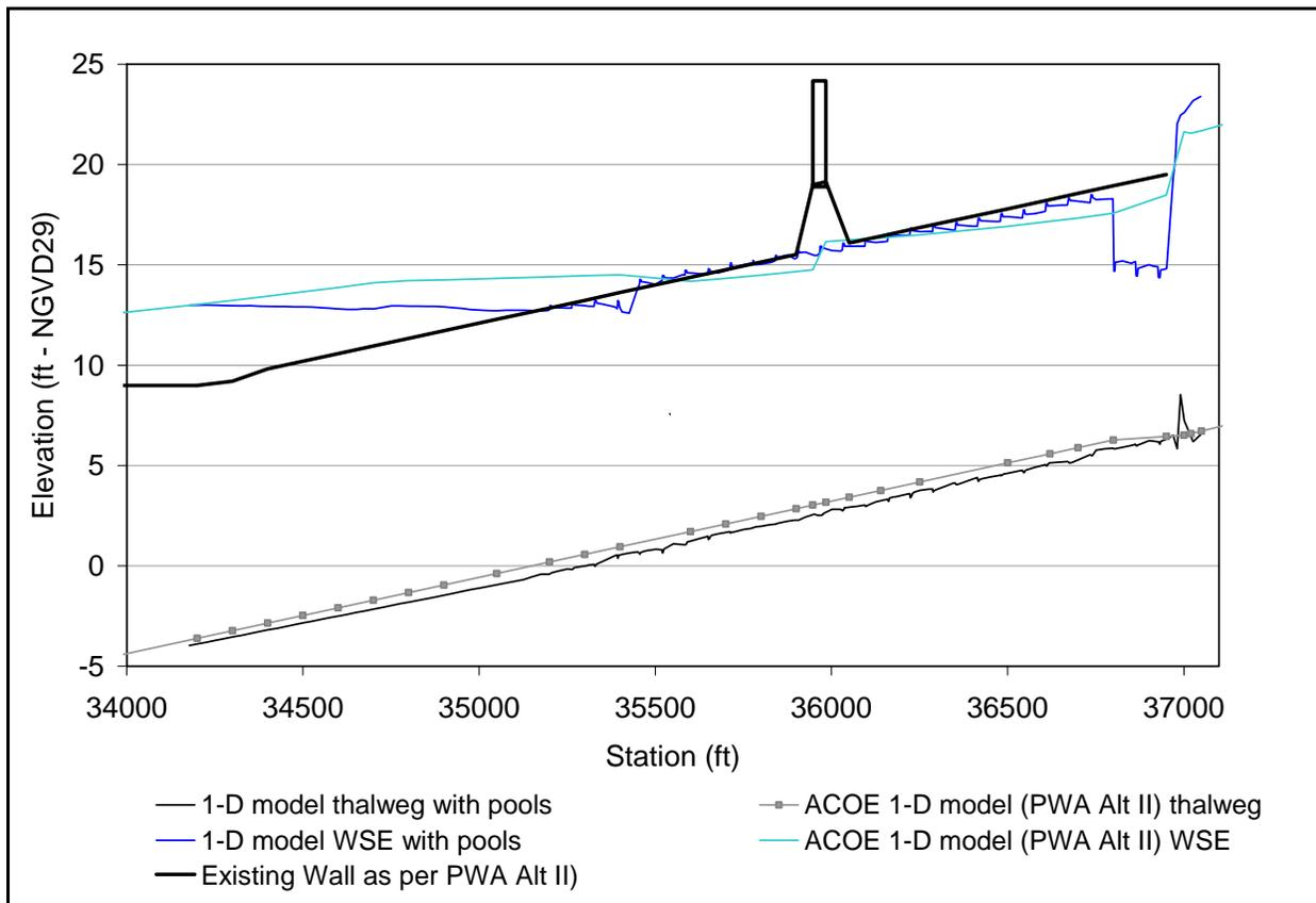
Figure 6.25 – Comparison of predicted water surface elevations for the 5,400 cfs target design flow for the 1-D model and the ACOE 1-D model.
