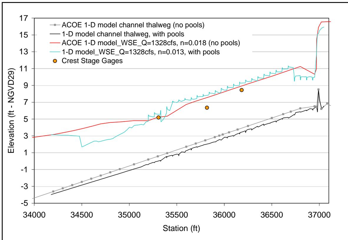
**Figure 6.24** – Comparison of water surface elevations predicted from 1-D models versus crest stage gage elevations at observed high flow of 1328 cfs on December 18, 2006.
