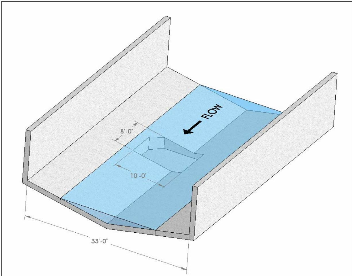
**Figure 6.12** – Isometric drawing of Alternative 2 resting pool.
