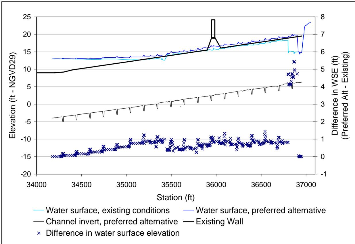
**Figure 6.26**– Comparison of predicted water surface elevations for the 5,400 cfs target design flow for existing conditions and the preferred pool alternative.
