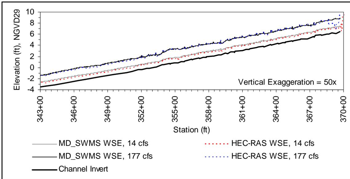
**Figure 4.1** - HEC-RAS and MD\_SWMS predictions of water surface elevation at 14 cfs and 177 cfs in model reach, Unit 3.
