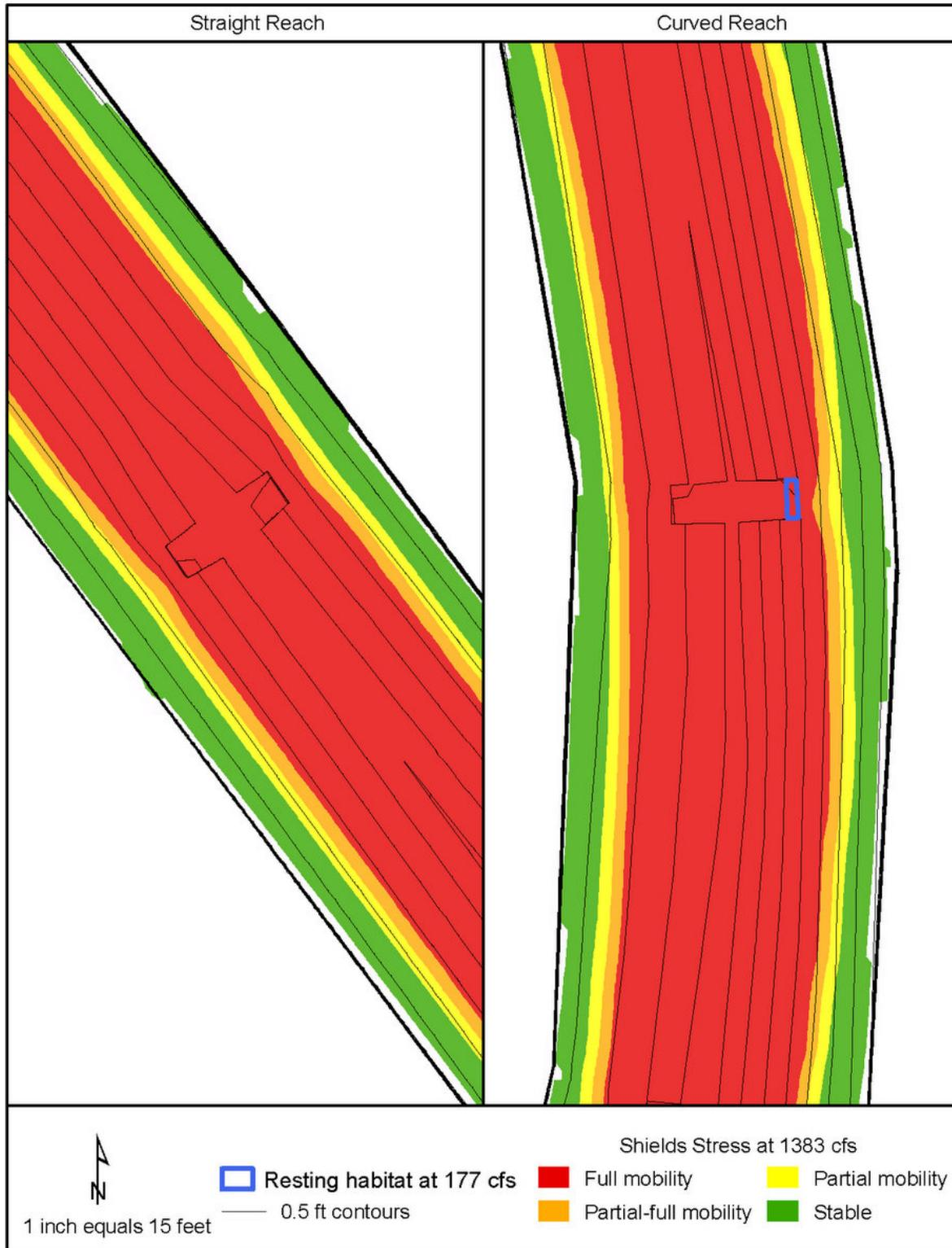
**Figure 6.5** – Existing predicted mobility of streambed material at the 1.5 year return flow of 1,383 cfs
