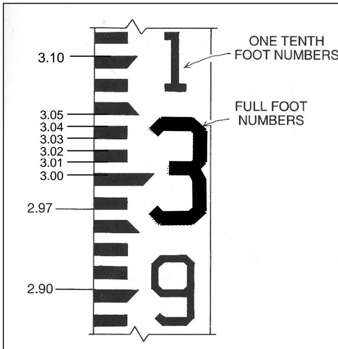
How to read a stage plate to the nearest 100<sup>th</sup> of a foot.
