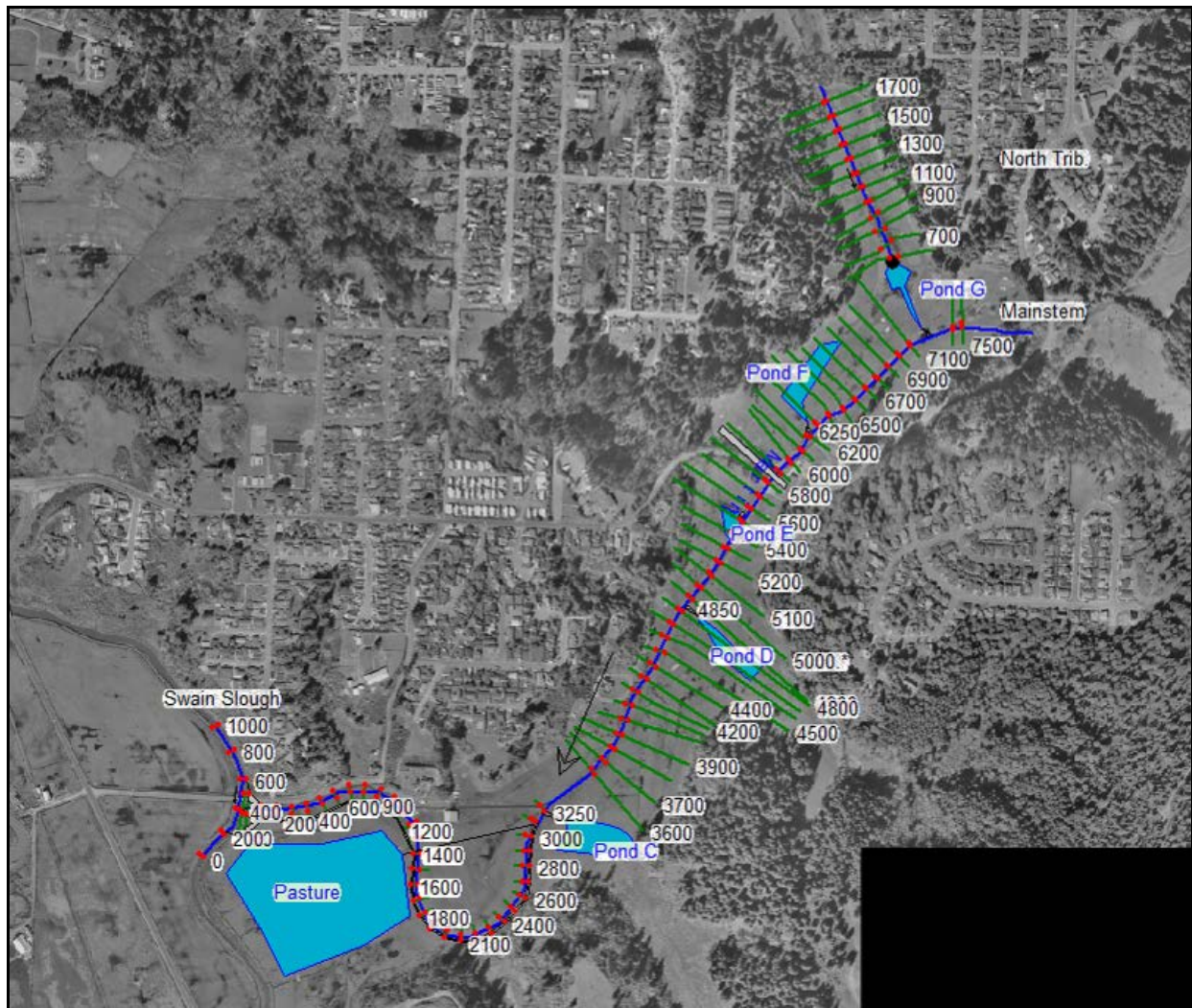
Figure 4-1. Schematic of HEC-RAS cross section locations (green) and storage areas (blue).
